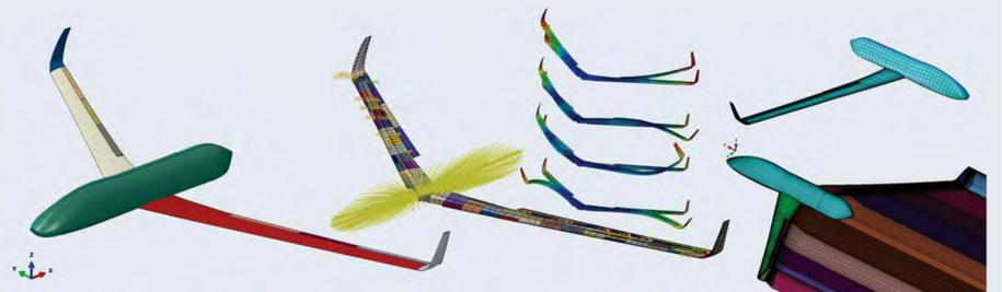
Only the wing is described by the structural model and the fuselage is considered by its inertial properties. The aeroelastic model is assembled using the first thirty modes of the FEM and the aerodynamic one is defined by about 20000 body elements. The total mass of the model is 4900 Kg.
