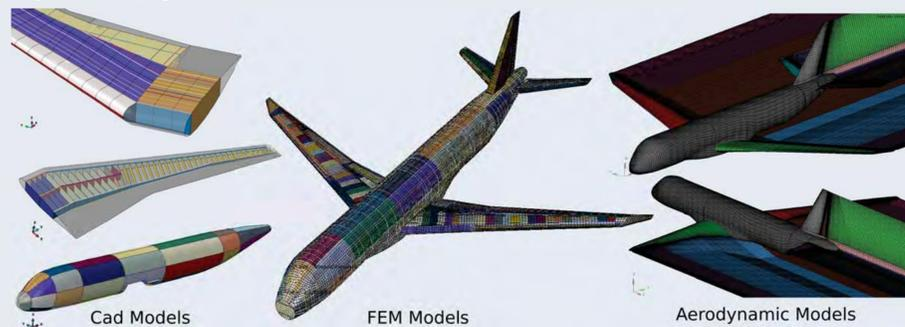
It is a Python object-oriented tool, developed taking advantages of Abaqus-CAE API, able to define structural and aerodynamic models, as the one reported in the figure above, fully automatically. It is also able to handle the different structural property definitions of the FEM and to export a parametric structural model used as input for the optimization module (PySIZE).
